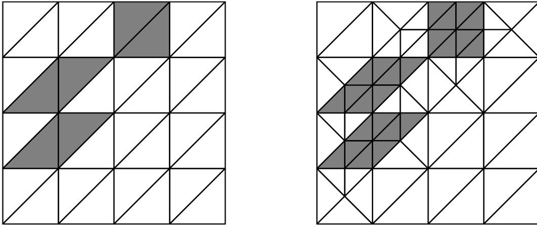
FIGURE 4.6. *The left plot shows an initial mesh  $\mathcal{T}_\ell$  with marked elements coloured in grey. The right plot shows the mesh  $\mathcal{T}_{\ell+1}$  obtained by RGB-refinement of the marked elements. The grey elements are obtained by uniform refinement of a marked element  $T \in \mathcal{T}_0$ .*
