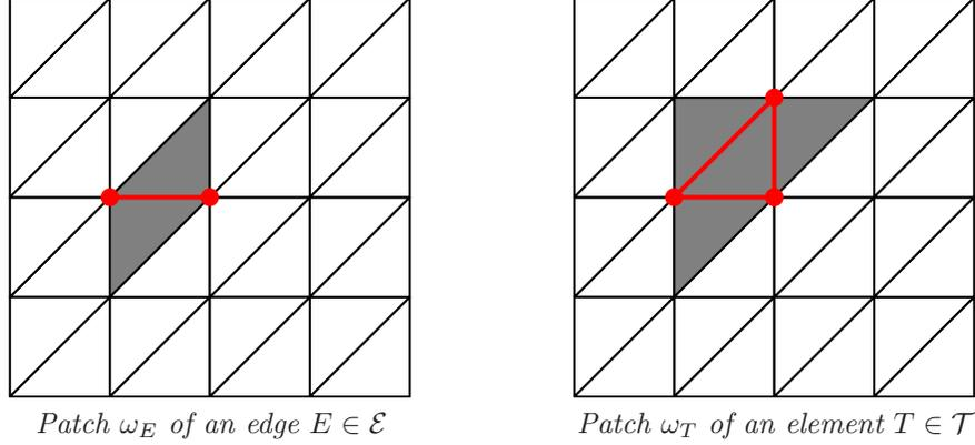
FIGURE 4.2. To prove the efficiency estimate, it suffices to consider smaller patches  $\omega_E \subseteq \Omega_E$  and  $\omega_T \subseteq \Omega_T$ , for edges  $E \in \mathcal{E}$  and elements  $T \in \mathcal{T}$ , respectively. For comparison with the larger patches  $\Omega_E$  and  $\Omega_T$ , the reader may consider Figure 4.1 on page 40.
