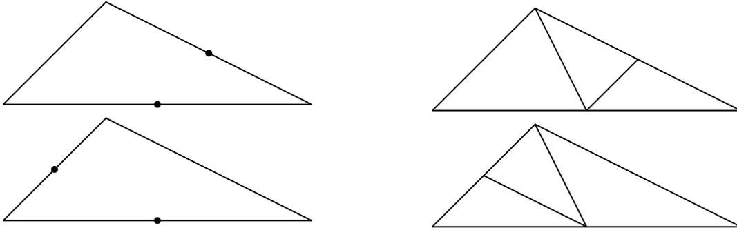
FIGURE 4.5. *Blue-refinement: If besides the longest edge of a triangle  $T \in \mathcal{T}_\ell$  just one other edge is marked for refinement (left),  $T$  is refined into three new triangles  $T_1, T_2, T_3 \in \mathcal{T}_{\ell+1}$  (right).*
