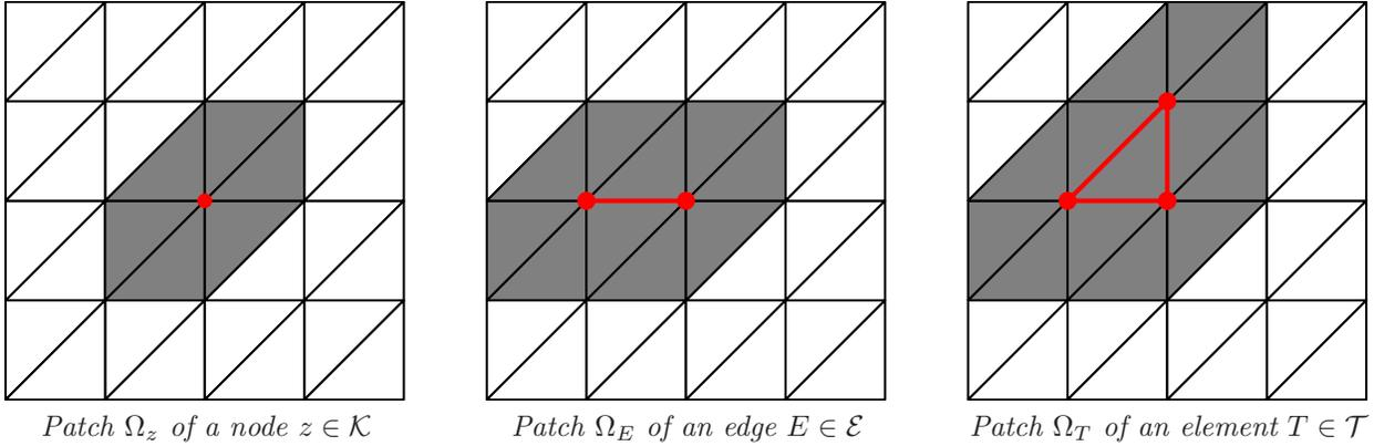
FIGURE 4.1. For the a posteriori analysis, we need three types of patches  $\omega \subseteq \Omega$ , namely patches of nodes, edges, and elements, respectively. Note that the patch of an edge (or of an element) just is the union of the patches of its nodes.
