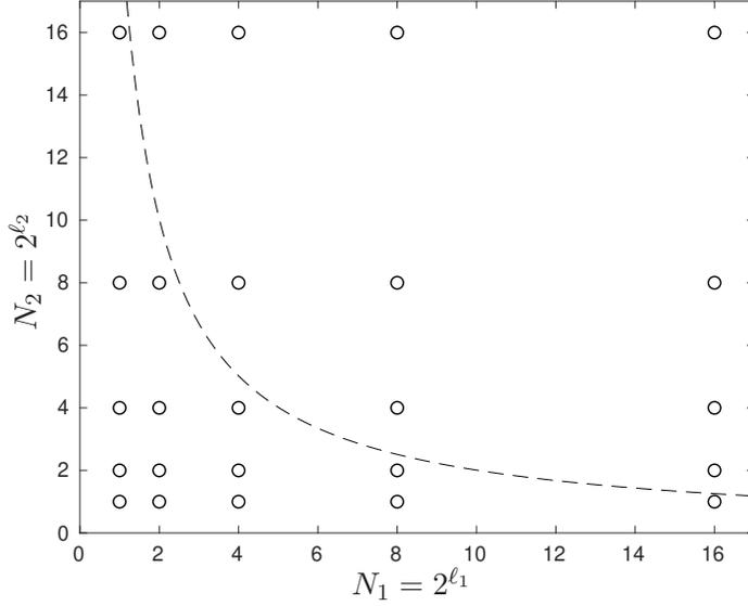
FIGURE 5.2. The circles represent the number of degrees of freedom of  $I_\ell$  in each coordinate direction. The sparse grid approach only uses interpolation operators which correspond to circles below the dashed line. This shape is the upper right quadrant of the so-called hyperbolic cross.
