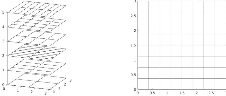
FIGURE 5.1. The different sparse grid contributions on the left stacked on top of each other combine to the full grid on the right. The interpolation operator  $I_{\ell} = I_{\ell_1}^{x_1} I_{\ell_2}^{x_2}$  corresponds to one of the grids on the left-hand side (e.g., grid number 1 for  $\ell = (1, 2)$  or grid number 5 for  $\ell = (3, 1)$ ).
