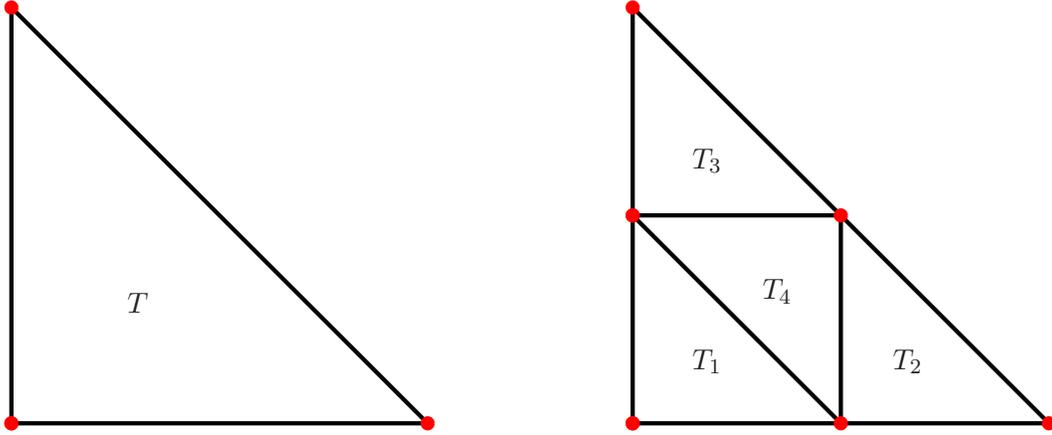
FIGURE 3.4. Red-refinement refines the element  $T \in \mathcal{T}^{(\text{old})}$  into 4 similar elements  $T_1, \dots, T_4 \in \mathcal{T}^{(\text{new})}$ . The new nodes  $\mathcal{K}^{(\text{new})} \setminus \mathcal{K}^{(\text{old})}$  are just the edge midpoints for all edges  $E \in \mathcal{E}^{(\text{old})}$ . In particular, regularity of  $\mathcal{T}^{(\text{old})}$  implies regularity of  $\mathcal{T}^{(\text{new})}$ .
